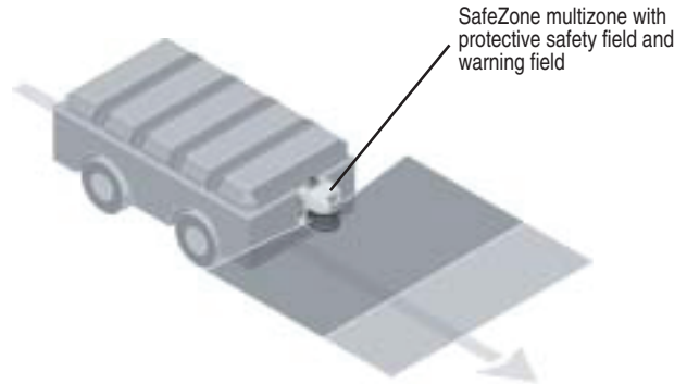
Figure 56: Vehicle monitoring with SafeZone safety laser scanner
